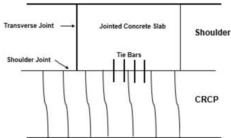
Figure 7. Diagram. Example of CRCP/JCP shoulder joint design.
