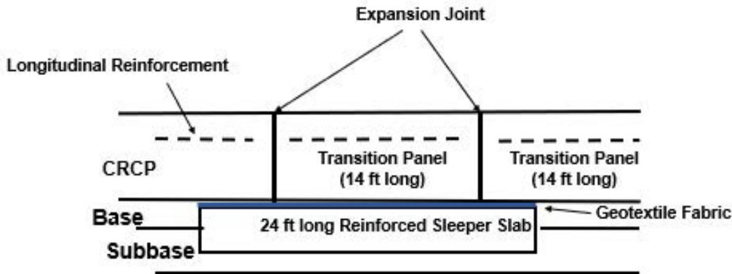
Figure 5. Diagram. Caltrans CRCP terminal joint design.
