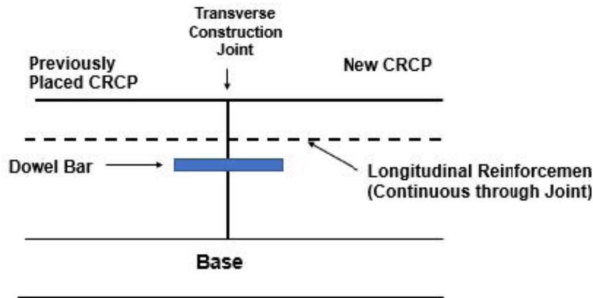
Figure 6. Diagram. Recommended CRCP transverse construction joint design.
