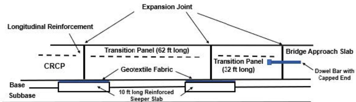
Figure 4. Diagram. Non-doweled CRCP terminal joint design.
